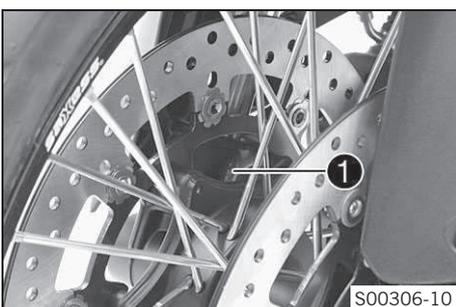
The fork part number ❶ is stamped on the inner side of the fork stub.
