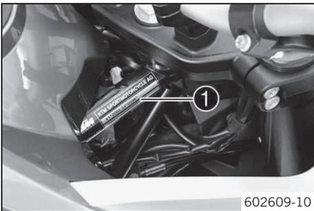
The type label ❶ is on the top right of the frame behind the steering head.
