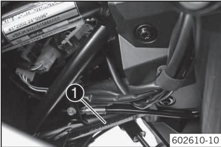
The chassis number ❶ is stamped on the bottom right of the frame behind the steering head.
