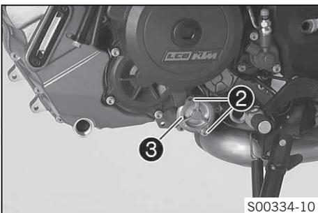
– Remove screws **2**. Remove the oil filter cover **3** with the O-ring.
