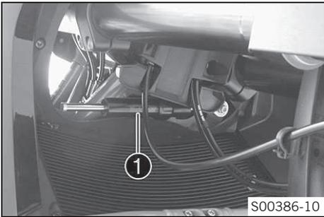
Steering damper item number ❶ is embossed on the underside of the steering damper.
